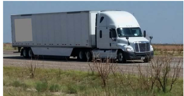
Figure 1. Test tractor-trailer on track in skirt-only configuration.
