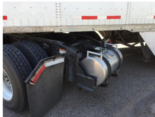
Figure 2. Example of weigh tank apparatus retrofitted to each tractor.
