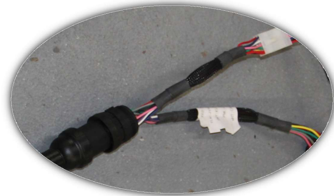
Figure 2. Backbone stub that gives each node access to the communication bus through the Molex 10-pin connector.
