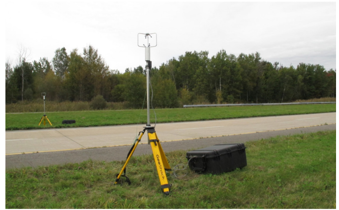
Figure 7. Track-side sonic anemometers.
