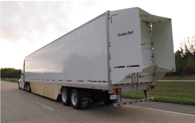
Figure 2. Photograph of the trailer configured with side-skirts and a boat-tail.
