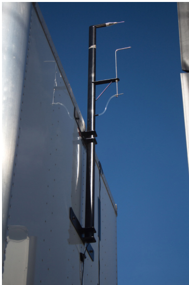
Figure 6. Wind-measurement probes mounted to front face of the trailer (velocity probe - high, pitot-static probe - low).
