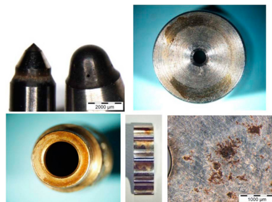
Figure 1. Different components of diesel fuel injection pumps with brown deposits on the surface: injection valve and spray nozzle, different metal rings (inlet piston /port of the fuel feed supply system), internal rotor and small part of a magnetic valve.
