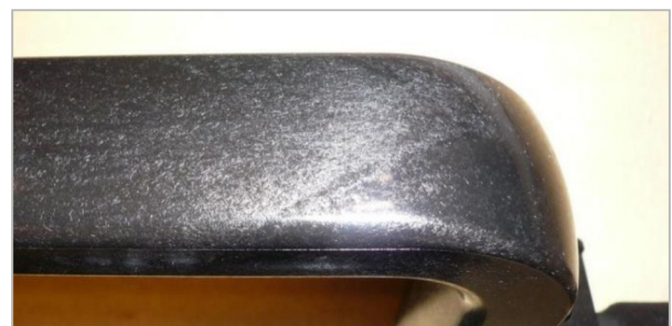
Figure 3. Surface appearance of a molded part of glass fiber reinforced resin (PPGF) by conventional injection molding
