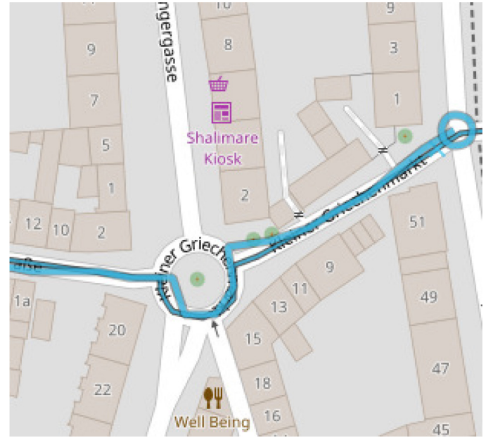
Figure 2. Illustration of Vehicle Agent trajectory with transparent erroneous vehicle position syncing back to solid true trajectory in the city of Cologne, Germany. Underlying map tile from OpenStreetMap.org
