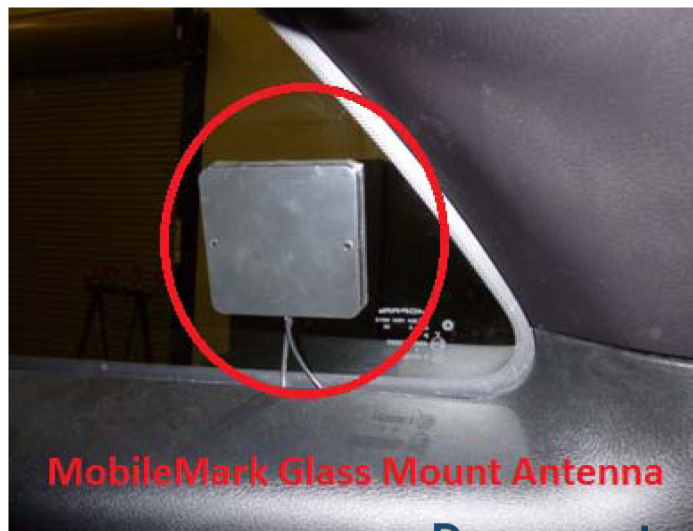
Fig. 2. Window DSRC Location
