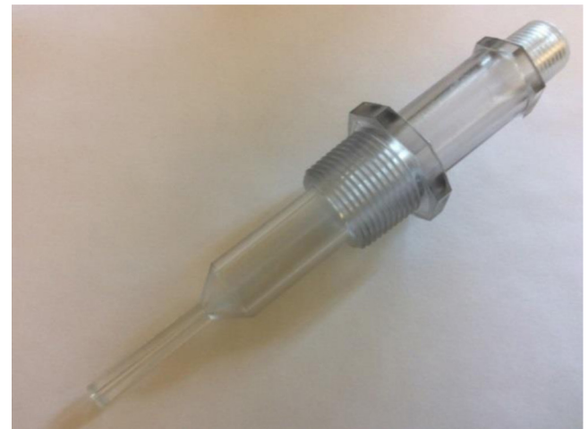
Figure 6. 3D printed transparent convergent-divergent nozzle.
