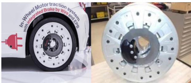
Figure 1. In-wheel motor assembled in the vehicle.
