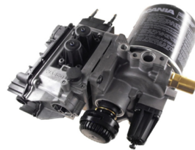
Figure 2. Photo of a new air dryer with desiccant cartridge on the top, control unit to the left and purge valve in the bottom.
