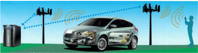
Figure 1. Implementation of MyFordMobile connectivity. This figure shows a customer communicating to his electrified vehicle, a Ford Focus Electric, through cellular technology. The customer connects to a Ford cloud-based secure server which in-turn communicates with his vehicle.
