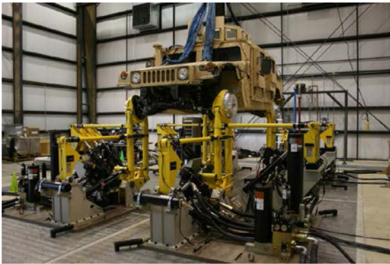
Figure 2. Spindle Coupled Vehicle Durability Simulator (VDS) at ATC.
