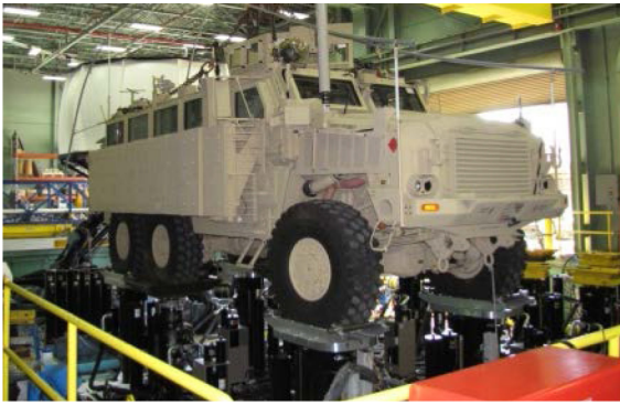
Figure 1. N-Post Simulator at TARDEC.
