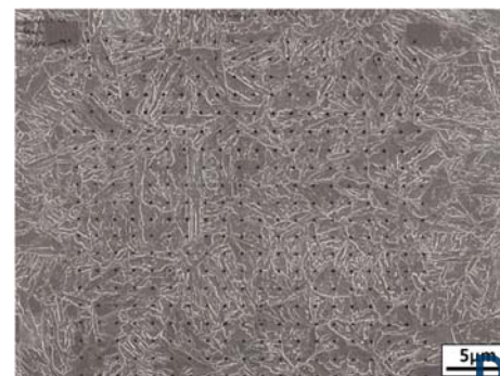
Figure 2. Overlay of indentation locations on SEM image of the etched Q&P steel.
