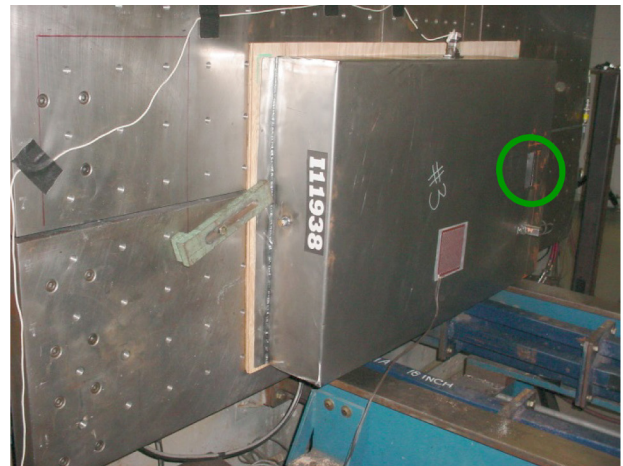
5b. Steel box with a RHS hole.
