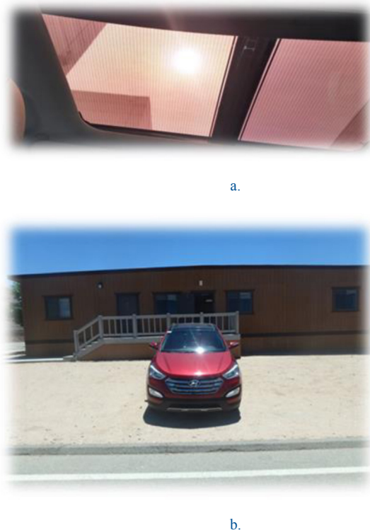
Figure 3. The photographs of (a) the semi-transparent solar roof taken from the inside vehicle, and (b) the solar power assisted automobile based on ‘Hyundai Santa Fe’w in HATCI.
