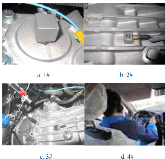
Figure 3. Vibration acceleration sensor and microphone sensor arrangements in experiments
