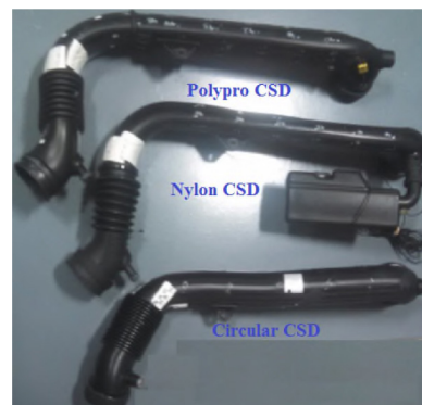
Figure 2. Three Test Clean Side Ducts
