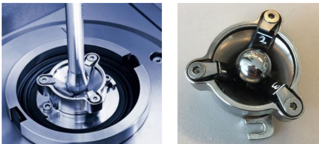
Figure 5. Ball-on-pyramid test set-up. The device used here is the commercially available Anton Paar Tribo-cell T-BTP installed in an Anton Paar MCR 501 Rheometer [3]. The left image shows the Tribo-cell installed in the rheometer and the right image the chromium steel ball (ISO 3290 G20) supported by 3 identical small plates of the material to be tested.
