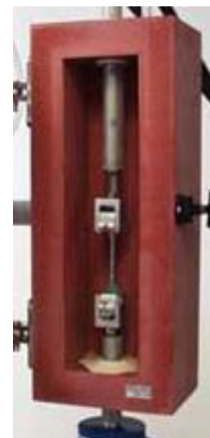
Figure 2. Tensile test setup used to derive failure strains.
