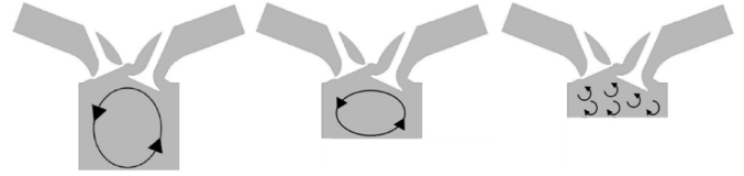
Figure 1. Illustration of the evolution of the tumble macro-vortex.
