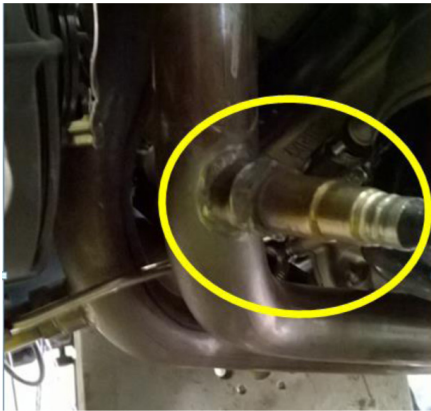
Figure 3. UEGO probe located in the exhaust runner
