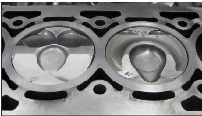
Figure 6. D-EGR high compression piston (left) compared to stock 9.3:1 piston (right).
