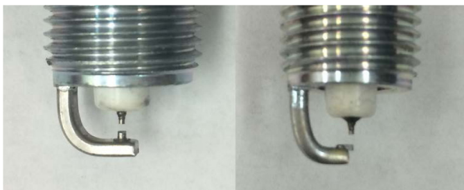
Figure 2. Left: double fine wire spark plug; Right: oval-J spark plug.
