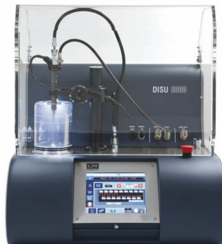
Figure 6. The injector test bench used by Laboratory 1
