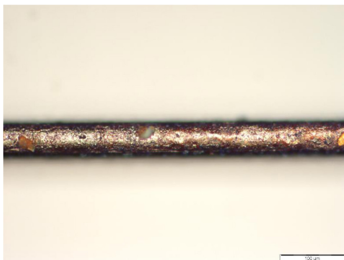
Figure 1. Optical microscope image of the end of test copper wire after 180 hours at 120 °C in commercial driveline lubricant L3.
