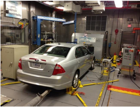
Figure 1. 2011 Ford Fusion test vehicle on APRF dynamometer for testing. Photo by Forrest Jehlik, Argonne National Laboratory
