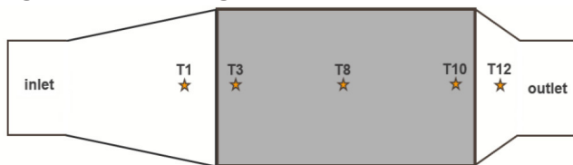
Figure 1. Representation of the thermocouples position. T1 and T12 measure the inlet and outlet gas temperatures respectively. The substrate temperatures are measured with the thermocouples T3, T8 and T10 mounted along the axis of the catalyst.
