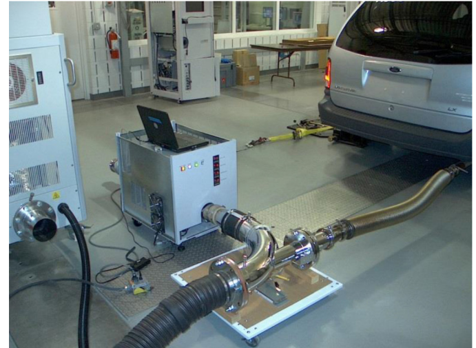
Figure 4. Configuration of the Ultrasonic Dilution Air Flow Meter test system in the chassis test cell. The conventional RMT (to the left of the ultrasonic flow meter) may be connected in series with the UFM to compare SSV and UFM dilution-air volume uncertainty.
