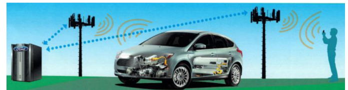
Figure 1. Implementation of MyFord Mobile connectivity. This figure shows a customer communicating to his electrified vehicle, a Ford Focus Electric, through cellular technology. The customer connects to a Ford cloud-based secure server which in-turn communicates with his vehicle [6].
