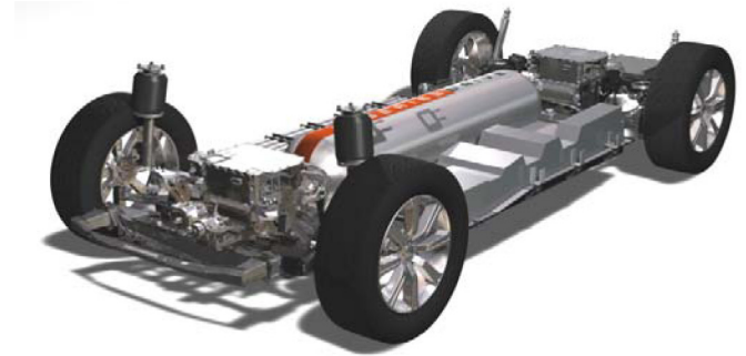
Figure 1. The baseline tank chosen for cost comparisons shown installed in a fuel cell vehicle platform (courtesy of Ford Motor Company).
