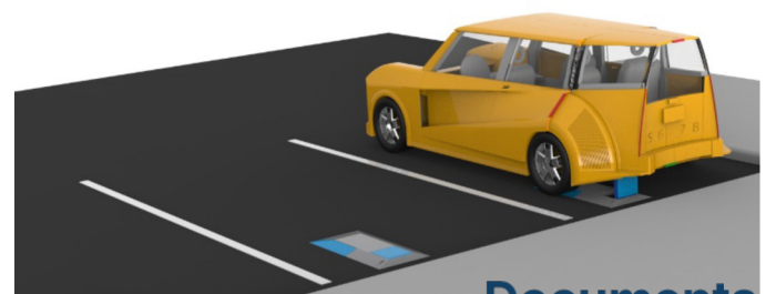
Figure 1. CAD model of desired compact, efficient, inductive solution [14]
