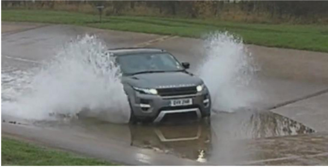
Figure 3. A Range Rover Evoque wading through water trough at a 50kph at Millbrook test facility. High amount of splashing is observed.
