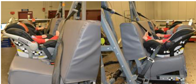
Figure 4. Carrier without base installations; left- standard seatbelt right-inflatable seatbelt installation
