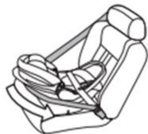
Figure 5. European seatbelt routing
