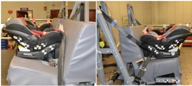
Figure 3. Carrier with base installations; left- standard seatbelt right-inflatable seatbelt installation
