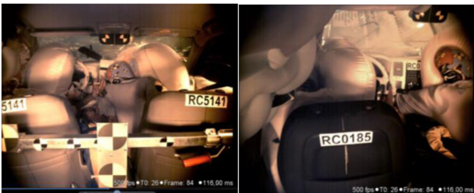
Figure 4. Examples of OI dummy kinematics shown at rebound time 116 ms
