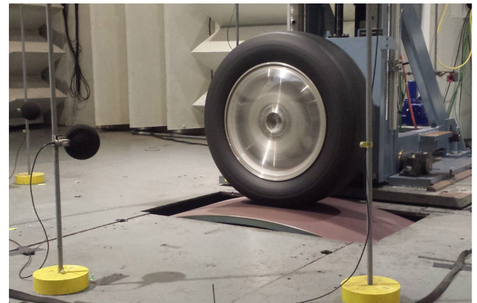
Figure 1. The experimental setup inside the semi-anechoic chamber located at Bridgestone Americas Technical Center in Akron, Ohio.
