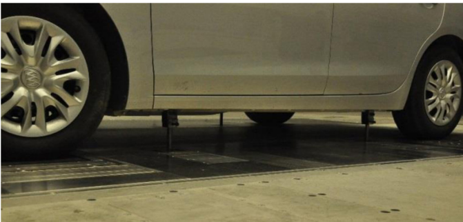
Figure 4. The vehicle was fixed to the wind tunnel floor by the struts clamped on the rocker-panel.
