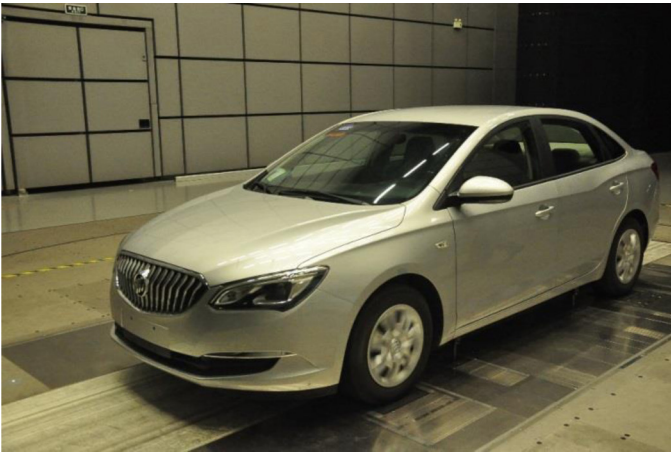
Figure 3. The vehicle and the moving belt system of the wind tunnel.
