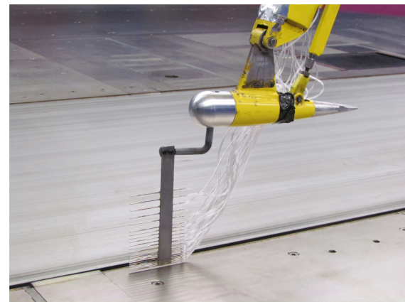
Figure 2. Boundary layer rake mounted on the traversing gear.
