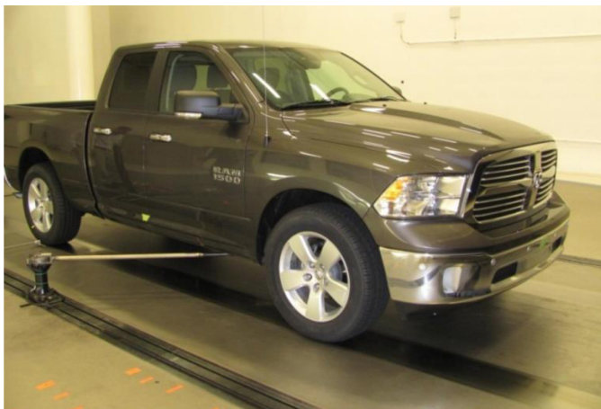
Figure 1. Ram 1500 in Windshear Wind Tunnel with Wheel design A
