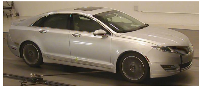
Figure 1. 2013 Lincoln MKZ test vehicle, shown here in a moving ground test condition.
