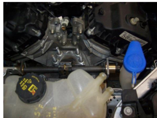
Figure 2. Engine translation mechanism, capable of moving the engine +/- 70mm for/aft.
