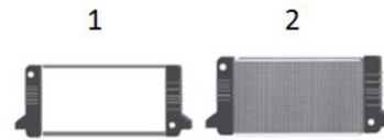
Figure 6. Condenser configurations, (1) without core, (2) with core.
