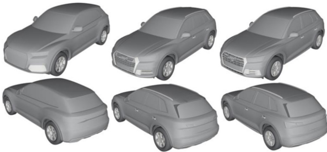
Figure 1. Evolution of vehicle design. left: design of 2012, middle: first 1:1 clay model, right: final car.
