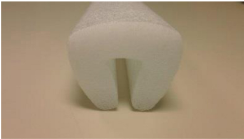
Figure 5. Styrofoam leading edge covering for the fan nacelle supports
