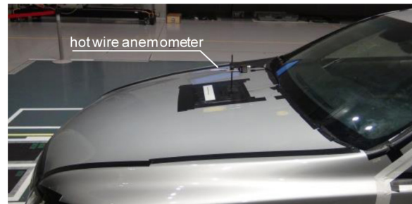
Figure 1. Hot wire anemometer mounted on hood
