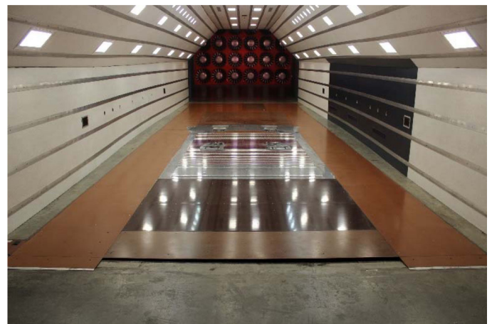
Figure 3. Wind tunnel working section (Courtesy: Aerodyn Technologies)
