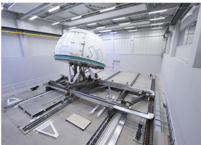
Figure 2. Stuttgart Driving Simulator with xy-table and hexapod (8 dof)
