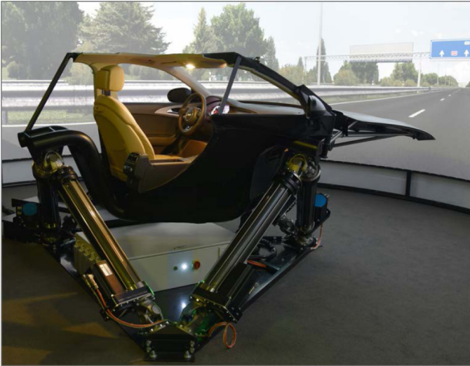
Figure 2. Cruden simulator used in this project
