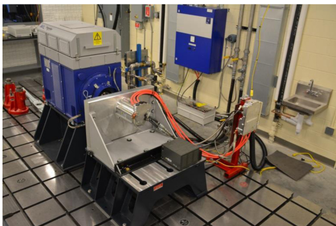
Figure 3. TM4 HSM 120 motor and CO150 motor control unit installed in ORNL's VSI lab component test cell
