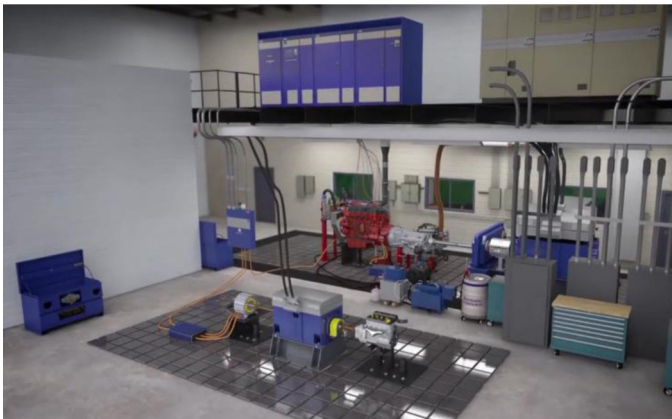
Figure 1. Rendering of the ORNL VSI laboratory test cells. The test cell used in this paper sits in the foreground but both cells share the battery emulator (blue cabinet) on the mezzanine
