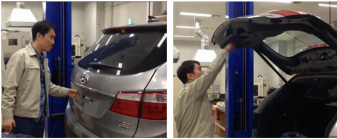
Figure 3. Knocking gestures to open or close the tailgate
