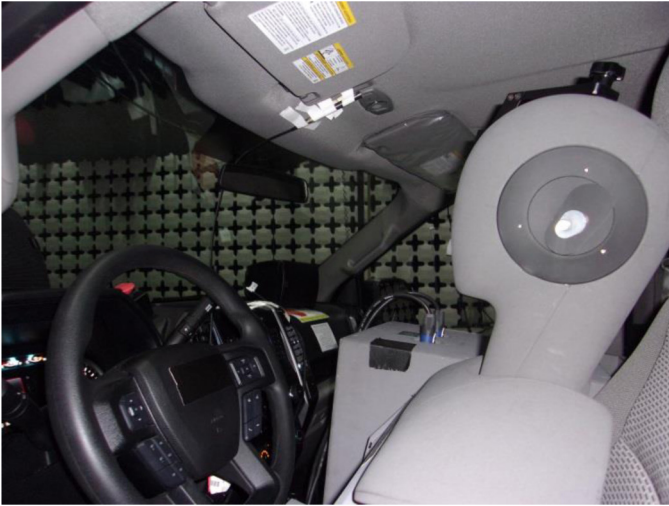
Figure 1. Example of the head and torso simulator in a vehicle to measure the cabin impulse response from the speaker's mouth to the cabin microphone location.
