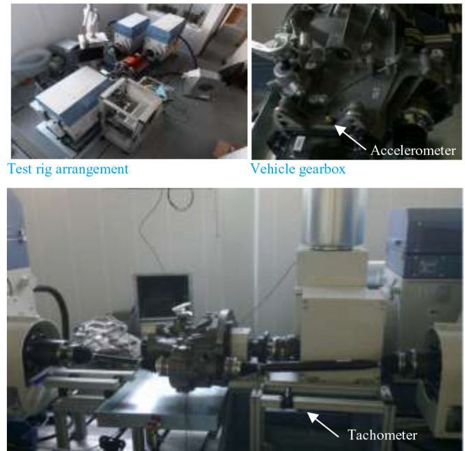
Figure 1. The open loop test bed used for investigation of faults in an automotive gearbox.
