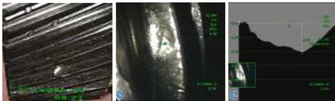
Figure 3. Detail of the pitting damaged created on one tooth only.
