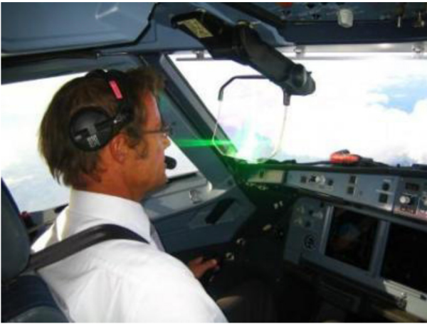
Figure 1. Avionics HUD: Overhead projection unit and combiner in front of the eyes (Source: THALES Avionics Onboard blog).
